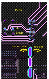
Figure 3 sense+/- layout example
