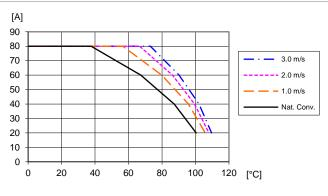
Available load current vs. ambient air temperature and airflow at Vı = 12 V.
