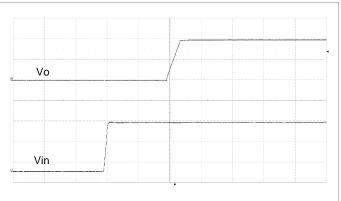
Output enabled by applying V<sub>I</sub>. V<sub>I</sub> = 12 V, I<sub>O</sub> = max I<sub>O</sub>. TON\_DELAY =0ms, TON\_RISE = 5 ms Scale top: 0.5 V/div, Scale bottom: 5V/div, time scale: 10 ms/div.
