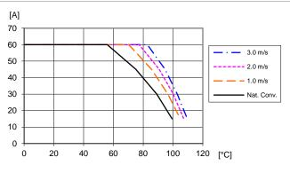
Available load current vs. ambient air temperature and airflow at  $V_{\rm I}$  = 12 V.
