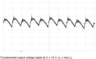
Fundamental output voltage ripple at V<sub>1</sub> = 12 V, I<sub>0</sub> = max I<sub>0</sub>,  $C_{OUT} = 10 \times 330 \ \mu\text{F}/10 \ m\Omega + 12 \times 100 \ \mu\text{F}$  Ceramic Scale: 2 mV/div, 1 µs/div, 20 MHz bandwidth. See section Output Ripple and Noise.
