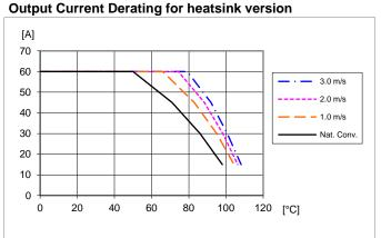
Available load current vs. ambient air temperature and airflow at  $V_1 = 12 V.$
