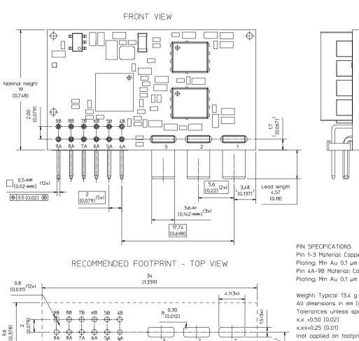
Pin 1-3 Material: Copper alloy (C11000) Plating: Min Au 0.1 µm over 1-3 µm Ni. Pin 4A-9B Material: Copper alloy Plating: Min Au 0.1 µm over 1 µm Ni.
