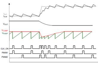
Figure 1 Load insertion response
