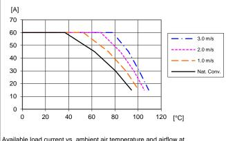
Available load current vs. ambient air temperature and airflow at Vı = 12 V.
