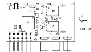
Temperature positions and air flow direction (Bottom side view)
