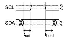
Setup and hold times timing diagram.
