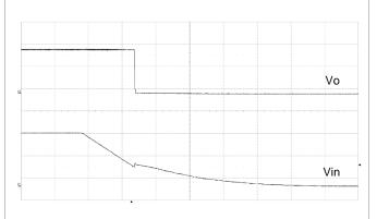
Output disabled by removing V<sub>I</sub>. V<sub>I</sub> = 12 V, I<sub>O</sub> = max I<sub>O</sub>. Scale top: 0.5V/div, scale bottom: 5V/div, time scale: 5 ms/div.
