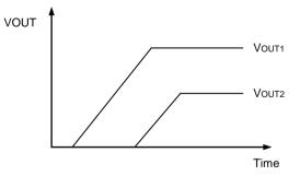
Illustration of Output Voltage Sequencing.
