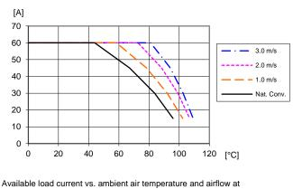
Available load current vs. ambient air temperature and airliow at  $V_1 = 12$  V.
