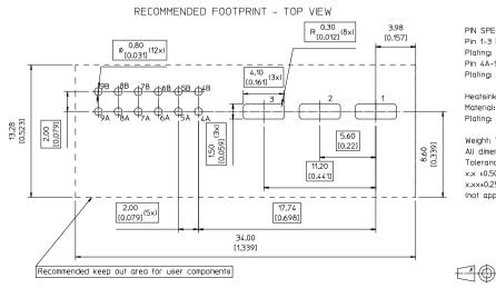
PIN SPECIFICATIONS Pin 1-3 Material: Copper alloy (C11000) Plating: Min Au 0.1 µm over 1-3 µm Ni. Pin 4A-9B Material: Copper alloy Plating: Min Au 0.1 µm over 1 µm Ni.
