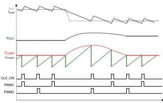
Figure 2 Load release response
