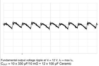
$C_{OUT} = 10 \times 330 \ \mu F/10 \ m\Omega + 12 \times 100 \ \mu F$  Ceramic Scale: 2 mV/div, 1 µs/div, 20 MHz bandwidth. See section Output Ripple and Noise.
