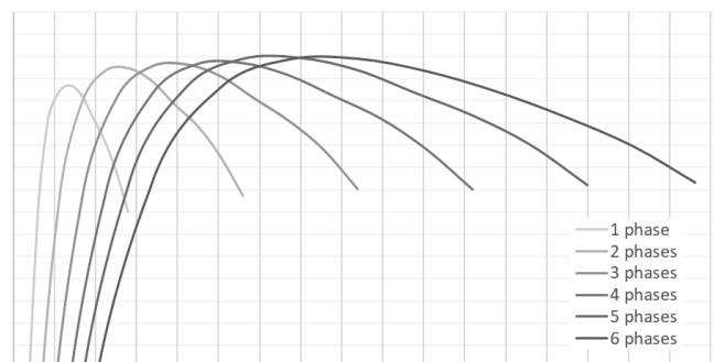
Illustration of efficiency vs load and number of active phases.
