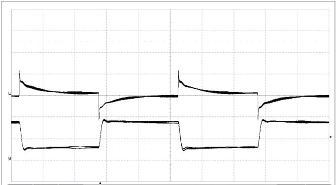
Output voltage response to load current step-
