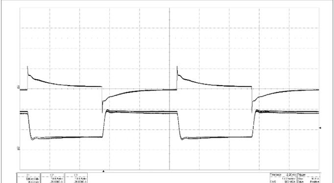
Output voltage response to load current step-
