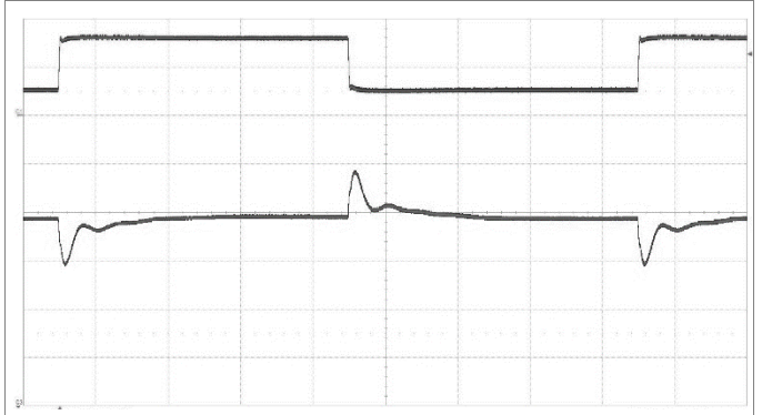
Output voltage response to load current step- change 27-81-27 A (2 A/ \mu\text{s} ) at: T_{PI} = +25^\circ\text{C} , V_i = 54\text{ V} . Top trace: load current 50 A/div. Bottom trace: output voltage 500 mV/div. Time scale: 0.5 ms/div.
