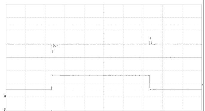
Output voltage response to load current step-
