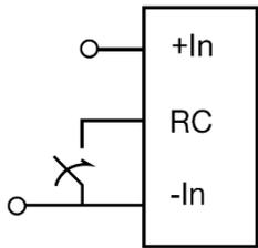
The products are fitted with a remote control function referenced to the primary negative input connection (-In), with negative logic options available. The RC function allows the product to be turned on/off by an external device like a semiconductor or mechanical switch.
