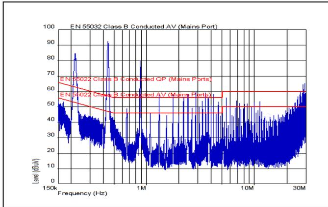
EMI without filter. EN55032 Test method and limits are the same as EN55022. 220  $\mu$ F 100V input capacitor and 2 x 1 mF 16 V OS-CON output capacitor used.
