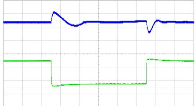
Output voltage response to load current step-
