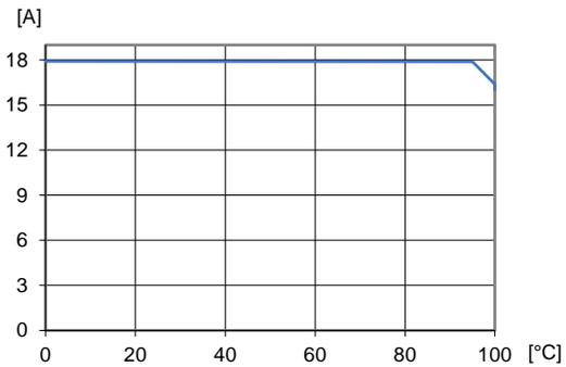
Available load current vs Base plate temperature.
