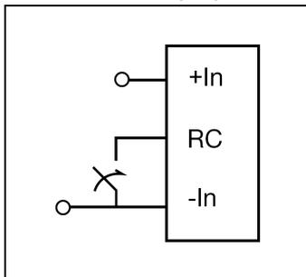
The products are fitted with a remote control function referenced to the primary negative input connection (-In), with negative and positive logic options available. The RC function allows the product to be turned on/off by an external device like a semiconductor or mechanical switch.
