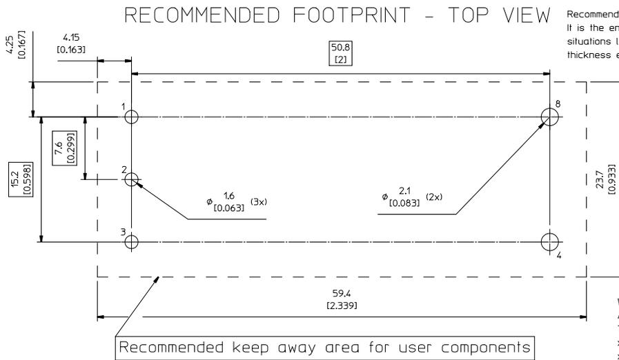
Recommended hole dimensions are only for reference. It is the end users decision based on different situations like production processes, substrate thickness etc.
