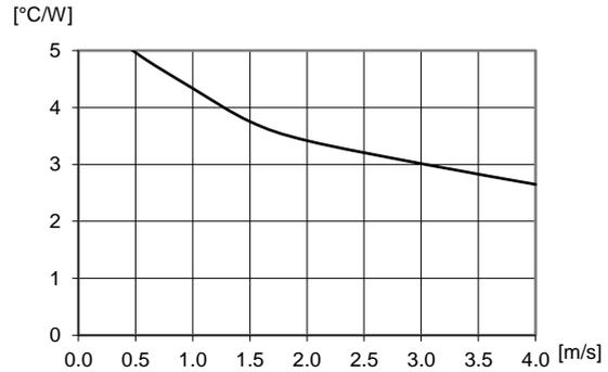
Thermal resistance vs. airspeed measured at the converter. Tested in wind tunnel with airflow and test conditions as per the Thermal consideration section.  $V_i = 24$  V.
