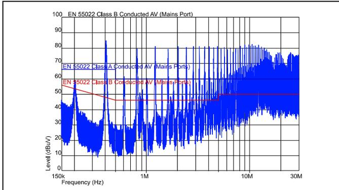
EMI without filter, EN55032 Test method and limits are the same as EN55022
