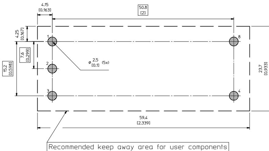
Recommended pad dimensions are not for reference. It is the end users decision based in different situations like production processes, substrate thickness etc.
