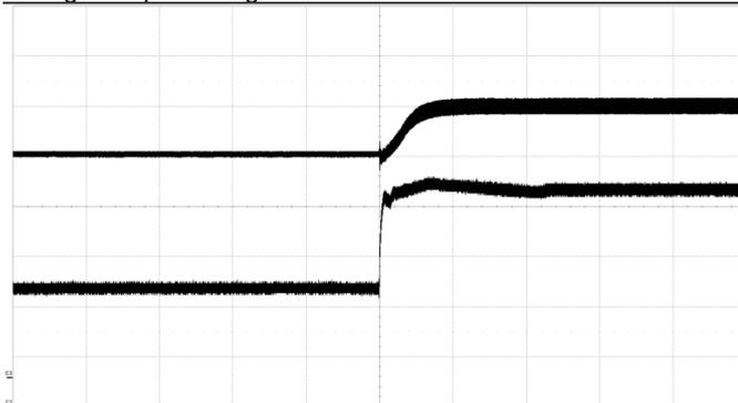
HRR product output at input voltage step 36-75 V, 1 ms/div
