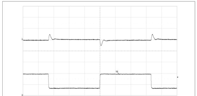
Output voltage response to load current step-change (6.25 – 18.75 – 6.25 A) at:
