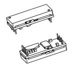
CASE Material: Aluminium For screw attachment apply mounting torque of max 0.44 Nm (3.9 lbf in). M3 screws must not protrude more than 3 mm [0.118] in to the base plate.
