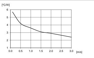
Thermal resistance vs. airspeed measured at the converter. Tested in wind tunnel with airflow and test conditions as per the Thermal consideration section.  $V_1 = 48 V$ .
