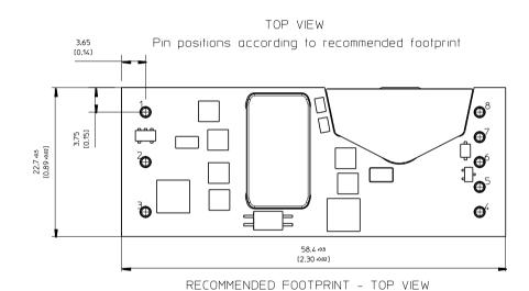
PIN SPECIFICATIONS Pin 1-8 Material: Copper alloy Plating: Min 0.1 μm Au over 1-3 μm Ni.
