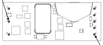
Pin 4 for measurement of minimum pin (solder joint) temperature, T<sub>PIN</sub>
