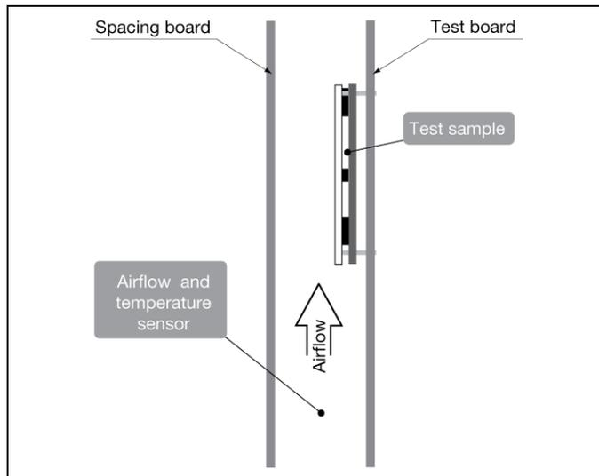
For products with baseplate used in a sealed box/cold wall application, cooling is achieved mainly by conduction through the cold wall. The Output Current Derating graphs are found in the Output section for each model. The product performance has been tested in a sealed box presented in the figure below. The ambient temperature (inside the box) has been set to 85°C. The cold wall temperature varied. See Design Note 028 for further details.
