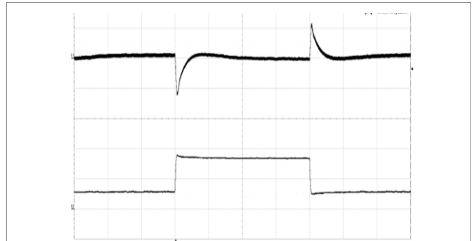
Output voltage response to load current step- change (1.125-3.375-1.125 A) at: T_{P1} = +25^{\circ}\text{C} , V_I = 24\text{ V} , dI/dt = 1\text{ A}/\mu\text{s} C_O = 22\text{ }\mu\text{F} ceramic capacitor Top trace: output voltage (200 mV/div.). Bottom trace: load current (2 A/div.). Time scale: (0.5 ms/div.).
