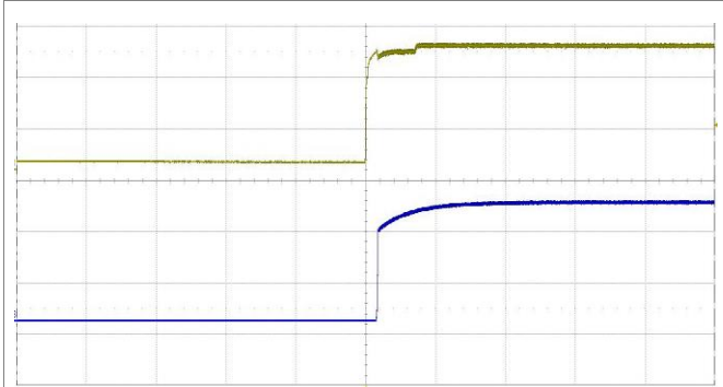
Start-up enabled by connecting V_I at: T_{P1} = +25^\circ\text{C} , V_I = 24\text{ V} , I_O = 2.5\text{ A} resistive load. Top trace: output voltage (10 V/div.). Bottom trace: input voltage (10 V/div.). Time scale: (50 ms/div.).
