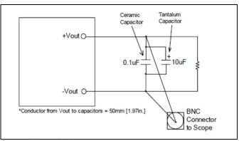
Output ripple and noise test setup
