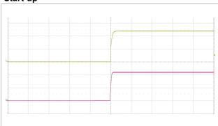
Start-up enabled by connecting  $V_{I}$  at:  $T_{P1}$  = +25°C,  $V_{I}$  = 110 V,  $I_{O}$  = 1.25 A resistive load. Top trace: output voltage (10 V/div.). Bottom trace: input voltage (50 V/div}). Time scale: (200 ms/div.).
