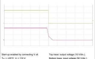
$T_{P1} = +25$ °C,  $V_I = 110$  V,  $I_O = 1.25$  A resistive load.
