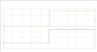
Start-up enabled by connecting V<sub>I</sub> at: T<sub>P1</sub> = +25°C, V<sub>I</sub> = 110 V, I<sub>O</sub> = 0.555 A resistive load.
