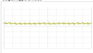
Output voltage ripple at: T<sub>P1</sub> = +25°C, VI = 110 V, I<sub>O</sub> = 6 A resistive load.
