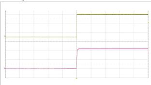
Start-up enabled by connecting V<sub>I</sub> at: T<sub>P1</sub> = +25°C, V<sub>I</sub> = 110 V, I<sub>O</sub> = 6 A resistive load.
