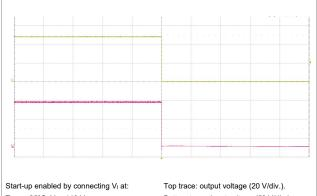
T<sub>P1</sub> = +25°C, V<sub>I</sub> = 110 V,  $I_0$  = 0.625 A resistive load. Bottom trace: input voltage (50 V/div.). Time scale: (200 ms/div.).
