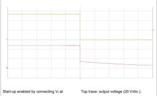
T<sub>P1</sub> = +25°C, V<sub>I</sub> = 110 V,  $I_0$  = 0.555 A resistive load. Bottom trace: input voltage (50 V/div.). Time scale: (200 ms/div.).
