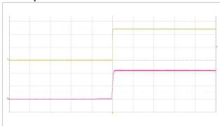
Start-up enabled by connecting V<sub>I</sub> at: T<sub>P1</sub> = +25°C, V<sub>I</sub> = 110 V, I<sub>O</sub> = 2.5 A resistive load.
