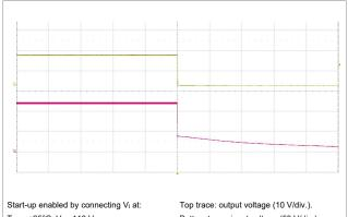
Start-up enabled by connecting V<sub>I</sub> at T<sub>P1</sub> = +25°C, V<sub>I</sub> = 110 V, I<sub>O</sub> = 2 A resistive load.
