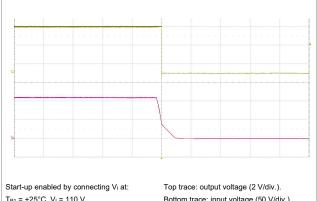
T<sub>P1</sub> = +25°C, V<sub>I</sub> = 110 V, Io = 6 A resistive load.
