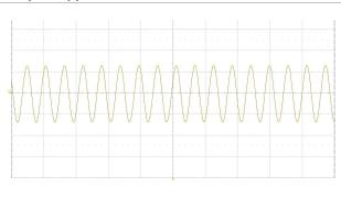
Output voltage ripple at: T<sub>P1</sub> = +25°C, VI = 110 V, I<sub>O</sub> = 0.555 A resistive load. Trace: output voltage (50 mV/div.). Time scale: (5 µs/div.). 20MHz bandwidth
