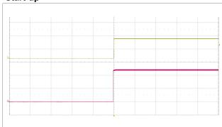
Start-up enabled by connecting  $V_I$  at:  $T_{P1}$  = +25°C,  $V_I$  = 110 V,  $I_O$  = 2 A resistive load. Top trace: output voltage (10 V/div.). Bottom trace: input voltage (50 V/div}). Time scale: (200 ms/div.).
