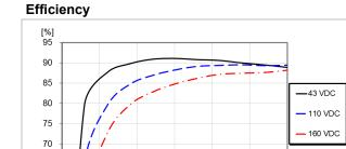
Efficiency vs. load current and input voltage at +25°C.
