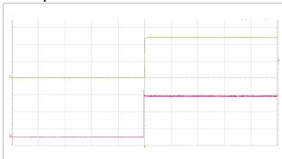
Start-up enabled by connecting V<sub>I</sub> at:  $T_{P1}$  = +25°C,  $V_{I}$  = 110 V, I<sub>O</sub> = 0.625 A resistive load.
