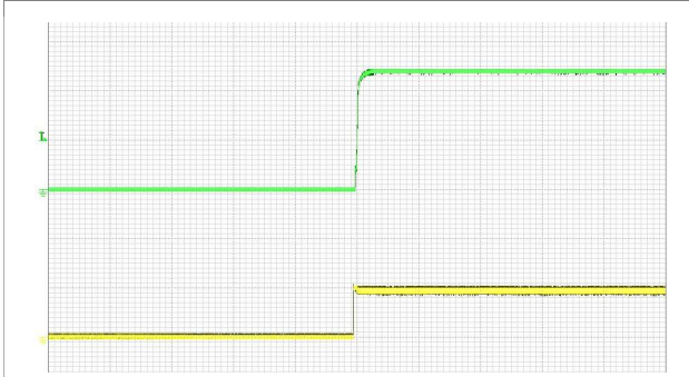
Start-up enabled by connecting V_i at: T_{P1} = +25^{\circ}\text{C} , V_i = 9\text{ V} , I_o = 8\text{ A} resistive load. Top trace: output voltage (20 V/div.). Bottom trace: input voltage (10 V/div.). Time scale: (100 ms/div.).
