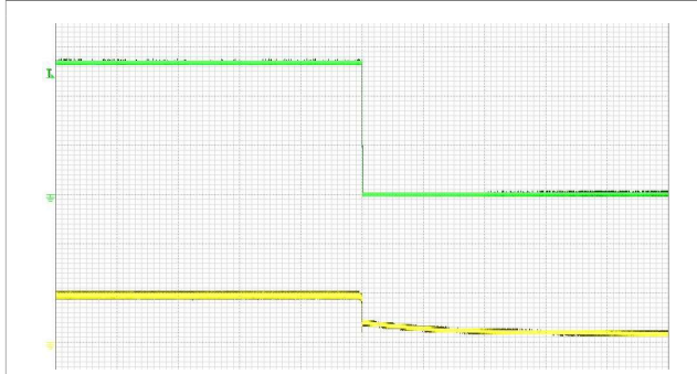
Start-up enabled by connecting V_i at: T_{P1} = +25^{\circ}\text{C} , V_i = 9\text{ V} , I_o = 0.74\text{ A} resistive load. Top trace: output voltage (20 V/div.). Bottom trace: input voltage (10 V/div.). Time scale: (100 ms/div.).
