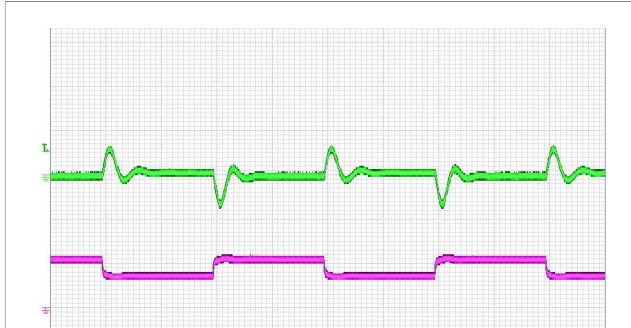
Output voltage response to load current step- change (0.37-0.555-0.37 A) at: T_{P1} = +25^{\circ}\text{C} , V_i = 48\text{ V} . Top trace: output voltage (1 V/div.). Bottom trace: load current (500 mA/div.). Time scale: (500 \mu\text{s} /div.).
