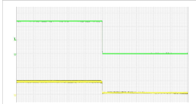
Start-up enabled by connecting V_i at: T_{P1} = +25^{\circ}\text{C} , V_i = 9\text{ V} , I_o = 0.83\text{ A} resistive load. Top trace: output voltage (20 V/div.). Bottom trace: input voltage (10 V/div.). Time scale: (100 ms/div.).
