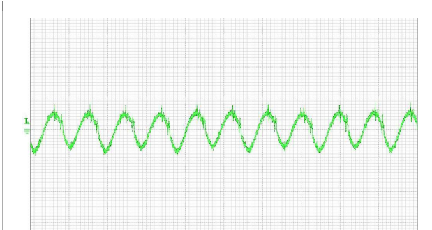
Output voltage ripple at: T_{P1} = +25^{\circ}\text{C} , V_i = 48\text{ V} , I_o = 1.67\text{ A} resistive load. Trace: output voltage (50 mV/div.). Time scale: (5 \mu\text{s} /div.). 20 MHz bandwidth
