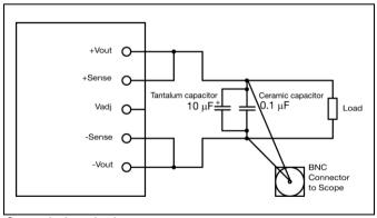
Output ripple and noise test setup
