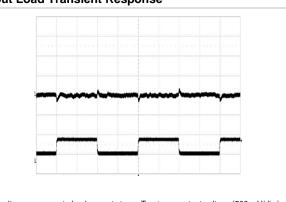
Output voltage response to load current step- Top trace: output voltage (500 mV/div.). change (3.5-10.5-3.5 A) at: T<sub>P1</sub> =+25°C, V<sub>I</sub> = 48 V.
