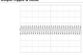
Output voltage ripple at:  $T_{P1} = +25$ °C,  $V_1 = 48$  V,  $I_0 = 14$  A resistive load.
