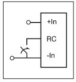
The products are fitted with a remote control function referenced to the primary negative input connection (-In), with negative and positive logic options available. The RC function allows the product to be turned on/off by an external device like a semiconductor or mechanical switch. The RC pin has an internal pull up resistor to +10V.
