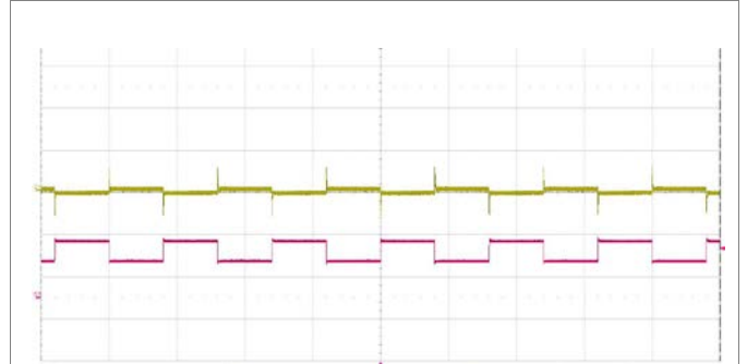
Output voltage response to load current step-change (6.66-10.0-6.66 A) at: T_{P1} = +25^{\circ}\text{C} , V_i = 110\text{ V} . Top trace: output voltage (500 mV/div.). Bottom trace: load current (5 A/div.). Time scale: (2 ms/div.).
