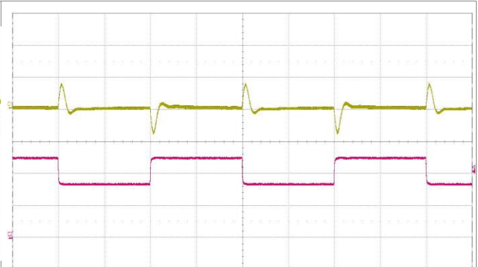
Output voltage response to load current step-change (8.4-12.5-8.4 A) at: T_{P1} = +25^\circ\text{C} , V_i = 36\text{ V} . Top trace: output voltage (500 mV/div.). Bottom trace: load current (5 A/div.). Time scale: (500 μs/div.).
