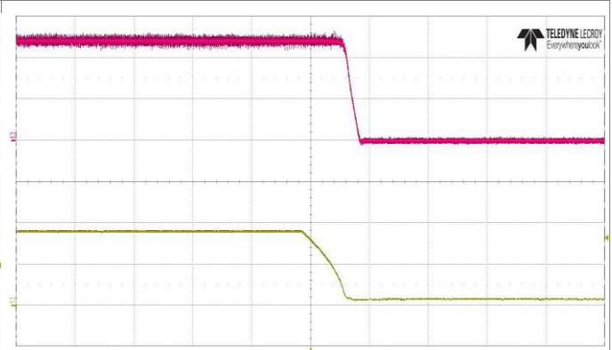
Shut-down enabled by disconnecting V_i at: T_{P1} = +25^\circ\text{C} , V_i = 36\text{ V} , I_o = 16.7\text{ A} resistive load. Top trace: output voltage (20 V/div.). Bottom trace: input voltage (5 V/div.). Time scale: (1 ms/div.).
