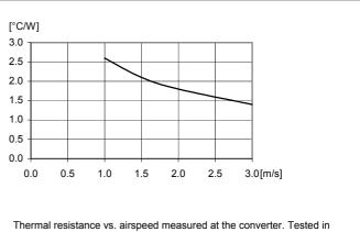
Thermal resistance vs. airspeed measured at the converter. Tested ir wind tunnel with airflow and test conditions as per the Thermal consideration section.  $V_1$  = 53 V.
