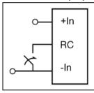
The products are fitted with a remote control function referenced to the primary negative input connection (-In), with negative and positive logic options available. The RC function allows the product to be turned on/off by an external device like a semiconductor or mechanical switch.
