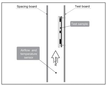
For products with base plate used in a sealed box/cold wall application, cooling is achieved mainly by conduction through the cold wall. The Output Current Derating graphs are found in the Output section for each module. The product is tested in a sealed box test set up with ambient temperatures 85 and 35°C. See Design Note 028 for further details.
