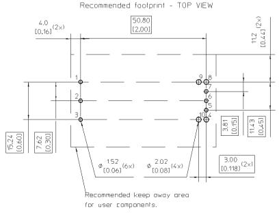
All dimensions are in mm [inches] Tolerances unless specified  $x.x \pm 0.5 \ [0.02]$
