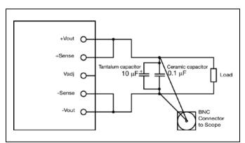
Output ripple and noise test setup
