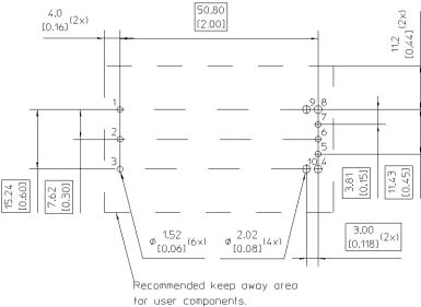
All dimensions are in mm [inches] Tolerances unless specified x.x ± 0.5 [0.02] x.xx ± 0.25 [0.01]
