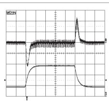
Output voltage response to load current step-change (3.75-11.25-3.37A) at  $T_{Pcb}$ =+25 °C, Vin=53 V. Top trace: output voltage (50mV/div.). Bottom trace: load current (5 A/div.) Time scale: 0.1 ms/div.
