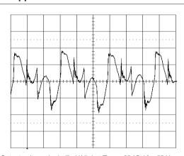
Output voltage ripple (5mV/div.) at  $T_{Pcb}$ =+25 °C, Vin=53 V, lo=20A resistive load with C=10  $\mu F$  tantalum and 0.1  $\mu F$  ceramic capacitors. Band width=20MHz. Time scale: 2 $\mu s$  / div.
