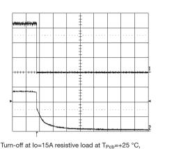
Turn-off at lo=15A resistive load at  $T_{Pcb}$ =+25 °C, Vin=53 V. Turn-off enabled by disconnecting Vin. Top trace: output voltage (1 V/div.). Bottom trace: input voltage (20 V/div.). Time scale: 10 ms/div.
