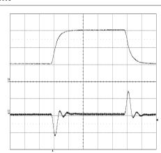
Output voltage response to load current step-change (5-15-5 A) at  $T_{Pcb}$ =+25 °C,  $V_{Pcb}$ =5 V. Top trace: load current (5 A/div.). Bottom trace: output voltage (100mV/div.) Time scale: 0.1 ms/div.
