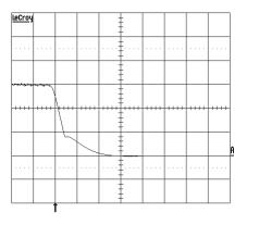
Turn-off at Io=10A resistive load at  $T_{Pcb}$ =+25 °C, Vin=53 V. Turn-off enabled by disconnecting Vin. Output voltage (0.5 V/div.). Time scale: 20 µs/div.
