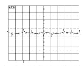
Output voltage ripple (50mV/div.) at  $T_{Pcb} = +25~^{\circ}C$ , Vin=53 V, Io=15A resistive load with C=10  $\mu F$  tantalum and 0.1  $\mu F$  ceramic capacitors. Band width=20MHz. Time scale: 1 $\mu s$  / div.
