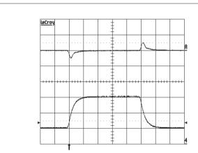
Output voltage response to load current step-change (5-15-5 A) at  $T_{Pcb}$ =+25 °C, Vin=53 V. Top trace: output voltage (200mV/div.). Bottom trace: load current (5 A/div.) Time scale: 0.1 ms/div.
