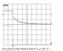
Turn-off at lo=20A resistive load at  $T_{Pcb}$ =+25 °C, Vin=53 V. Turn-off enabled by disconnecting Vin. Bottom trace: output voltage (0.5 V/div.). Top trace: input voltage (20 V/div.). Time scale: 5 ms/div.
