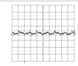
Output voltage ripple (50mV/div.) at  $T_{Pcb}$ =+25 °C, Vin=53 V, Io=10A resistive load with C=10  $\mu$ F tantalum and 0.1  $\mu$ F ceramic capacitors. Band width=20MHz. Time scale:  $2\mu$ 5 / div.
