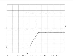
Start-up at Io=20A resistive load at  $T_{Pcb}$ =+25 °C, Vin=53 V. Start enabled by connecting Vin. Top trace: input voltage (20 V/div.). Bottom trace: output voltage (0.5 V/div.). Time scale: 5 ms/div.
