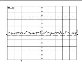
Output voltage ripple (50mV/div.) at  $T_{Pcb}{=}+25~^{\circ}C$ , Vin=53 V, Io=20A resistive load with C=10  $\mu F$  tantalum and 0.1  $\mu F$  ceramic capacitors. Band width=20MHz. Time scale:  $2\mu s$  / div.
