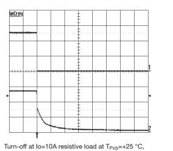
Turn-off at lo=10A resistive load at T<sub>Pcb</sub>=+25 °C, Vin=53 V. Turn-off enabled by disconnecting Vin. Top trace: output voltage (2 V/div.). Bottom trace: input voltage (20 V/div.). Time scale: 10 ms/div.
