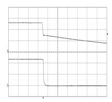
Turn-off at lo=20A resistive load at  $T_{Pcb}$ =+25 °C, Vin=53 V. Turn-off enabled by disconnecting Vin. Top trace: input voltage (20mV/div.). Bottom trace: Output voltage (0.5 V/div.). Time scale: 500 µs/div.
