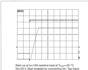
input voltage (10 V/div.). Bottom trace: output voltage
