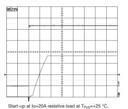
Start-up at Io=20A resistive load at  $T_{Pcb}$ =+25 °C, Vin=53 V. Start enabled by connecting Vin. Top trace: input voltage (10 V/div.). Bottom trace: output voltage (0.5 V/div.). Time scale: 5 ms/div.
