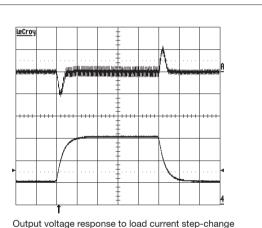
Output voltage response to load current step-change (5-15-5 A) at T<sub>Pcb</sub>=+25 °C, Vin=53 V. Top trace: output voltage (100mV/div.). Bottom trace: load current (5 A/div.) Time scale: 0.1 ms/div.
