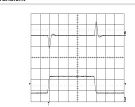
Output voltage response to load current step-change (3.75-11.25-3.75 A) at  $T_{Pcb}$ =+25 °C,  $V_{Pcb}$ =5 V. Top trace: output voltage (200mV/div.). Bottom trace: load current (5 A/div.) Time scale: 0.1 ms/div.
