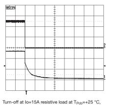
Turn-off at Io=15A resistive load at  $T_{Pcb}$ =+25 °C, Vin=53 V. Turn-off enabled by disconnecting Vin. Top trace: output voltage (1.0 V/div.). Bottom trace: input voltage (20 V/div.). Time scale: 10 ms/div.
