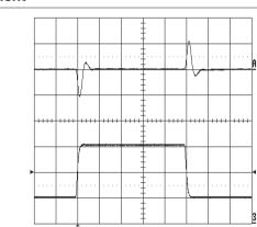
Output voltage response to load current step-change (2.5-7.5-2.5 A) at  $T_{Pcb}$ =+25 °C, Vin=53 V. Top trace: output voltage (200mV/div.). Bottom trace: load current (2.5 A/div.) Time scale: 0.1 ms/div.
