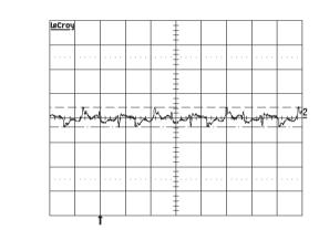
Output voltage ripple (50mV/div.) at  $T_{Pcb}{=}+25~^{\circ}C$ , Vin=53 V, lo=20A resistive load with C=10  $\mu F$  tantalum and 0.1  $\mu F$  ceramic capacitors. Band width=20MHz. Time scale:  $2\mu s$  / div.
