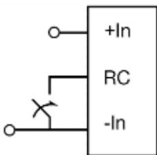
The products are fitted with a remote control function referenced to the primary negative input connection (-In), with negative and positive logic options available. The RC function allows the product to be turned on/off by an external device like a semiconductor, or a mechanical switch placed close to the product. The RC pin has an internal pull up resistor of 10 k $\Omega$  to +5 V. The threshold level has a hysteresis and the function is designed to be robust to noise.
