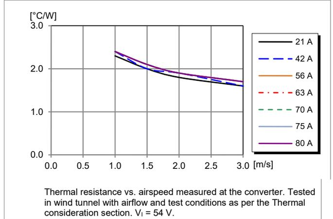
**Output Power Derating – Baseplate and 1/2" heat sink**
