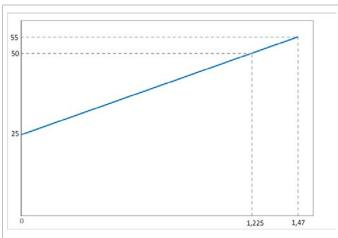
Desired output voltage vs. adjust voltage, Radj =  $0 \text{ k}\Omega$
