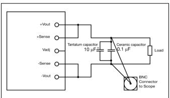
Output ripple and noise test setup
