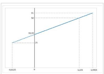
Desired output voltage vs. adjust voltage, Radj = 1 k $\Omega$
