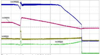
Blue line – output voltage peak at 11.3 V, 1 V/div Red line – input voltage change 54-44-72 V, 20 V/div
