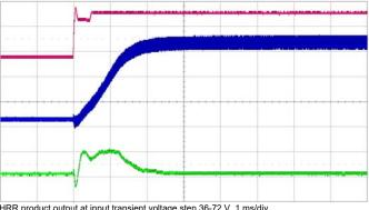
HRR product output at input transient voltage step 36-72 V, 1 ms/div Red line – input voltage change 36-72 V, 20 V/div Blue line - resulting output voltage change, 1 V/div
