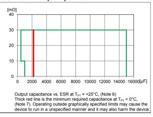
Note 6: ESR include conductor resistance between capacitor and output pins of the device Note 7: 2200 µF will satisfy load requierments during start-up and is only needed if application is required to perform start-up in cold environments.
