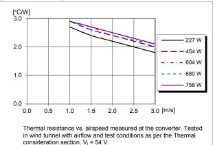
Thermal Resistance – Dual pin and base plate (PKM 4717 NH PI HS)
