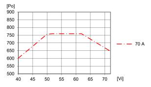
To enable a high power capability at low input voltages the input under voltage lockout is set to start the product when the input voltage reaches the typical value found in the Electrical Specification.
