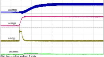
Red line – input voltage change 54-44-72 V, 20 V/div Yellow line –input current supplied from the HU- capacitor, 50 A/div
