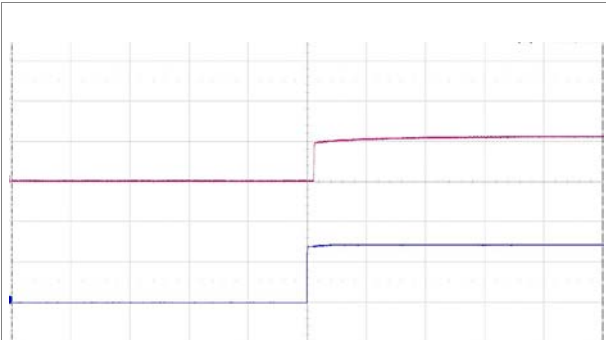
Start-up enabled by connecting V_I at: T_{P1} = +25^{\circ}\text{C} , V_I = 72\text{ V} , I_O = 0.95\text{ A} resistive load. Top trace: output voltage (50 V/div.). Bottom trace: input voltage (50 V/div.). Time scale: (50 ms/div.).
