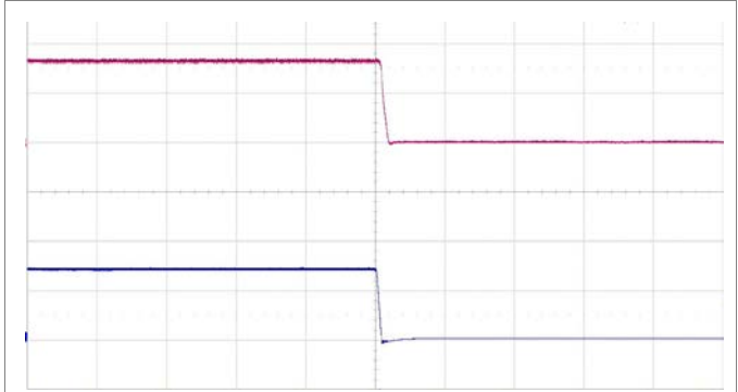
Shut-down enabled by disconnecting V_I at: T_{P1} = +25^\circ\text{C} , V_I = 72\text{ V} , I_O = 15.2\text{ A} resistive load. Top trace: output voltage (2 V/div.). Bottom trace: input voltage (50 V/div.). Time scale: (2 ms/div.).
