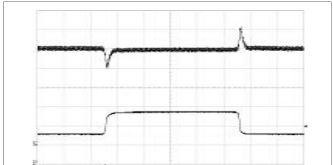
Output voltage response to load current step-change (6.25-18.75-6.25 A) at: T_{P1} = +25^\circ\text{C} , V_1 = 53\text{ V} . Top trace: output voltage (100 mV/div.). Bottom trace: load current (10 A/div.). Time scale: (0.1 ms/div.).
