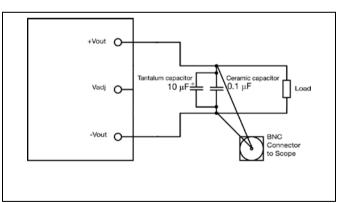
Output ripple and noise test setup
