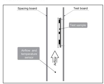
For products with gap-pad used in a sealed box/cold wall application, cooling is achieved mainly by conduction through the cold wall. The Output Current Derating graphs are found in the Output section for each model. The product is tested in a sealed box test set up with ambient temperatures 85 °C. See Design Note 028 for further details.
