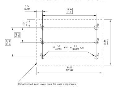
Recommended hale dimensions are only for reference. It is the end users decision based on different situations like production processes, substrate thickness etc.
