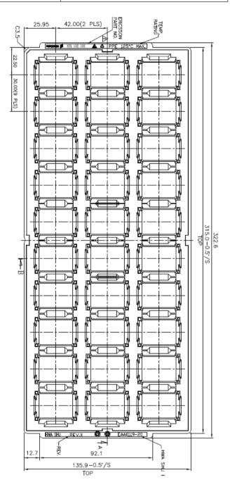
JEDEC standard tray for 3x10 = 30 products. All dimensions in mm [inch] Tolerances: X.x ±0.26 [0.01], X.xx ±0.13 [0.005] Note: pick up positions refer to center of pocket. See mechanical drawing for exact location on product.
