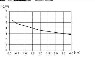
Thermal resistance vs. airspeed measured at the converter. Tested in wind tunnel with airflow and test conditions as per the Thermal consideration section.  $V_1 = 53 \ V$ .
