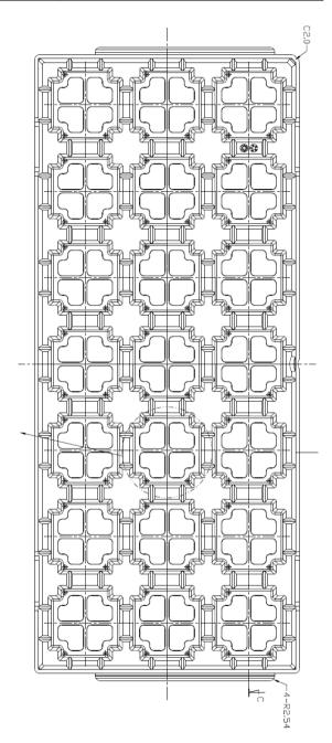
JEDEC standard tray for 2x10 = 20 products. All dimensions in mm [inch] Tolerances:  $X.x \pm 0.26$  [0.01],  $X.xx \pm 0.13$  [0.005] Note: pick up positions refer to center of pocket. See mechanical drawing for exact location on product.
