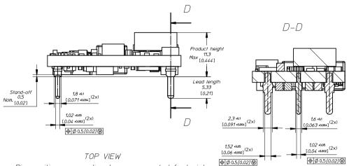
Pin positions according to recommended footprint
