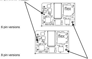
Pin 4 for measurement of minimum pin (solder joint) temperature, T<sub>PIN</sub>
