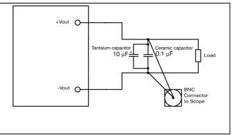
Output ripple and noise test setup
