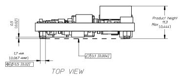
Pin position according to the recommended footprint
