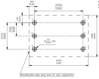
Recommended pad dimensions are only for reference. It is the end users decision based on different situations like production processes, substrate thickness etc.
