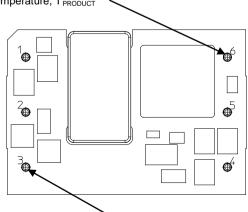
Pin 3 for measurement of minimum pin (solder joint) temperature, T<sub>PIN</sub>
