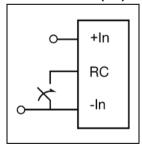
The products are fitted with a remote control function referenced to the primary negative input connection (-In), with negative and positive logic options available. The RC function allows the product to be turned on/off by an external device like a semiconductor or mechanical switch. The RC pin has an internal pull up resistor.
