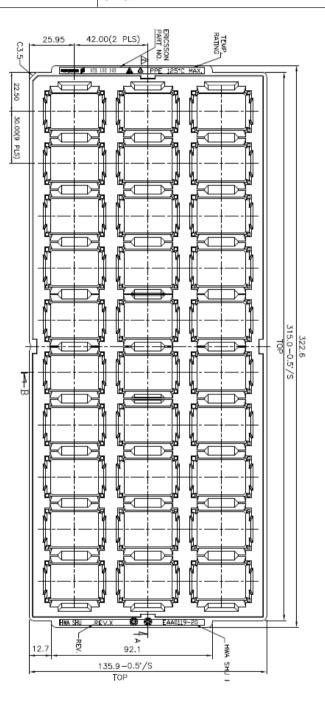
JEDEC standard tray for 3x10 = 30 products. All dimensions in mm [inch] Tolerances:  $X.x \pm 0.26 [0.01]$ ,  $X.xx \pm 0.13 [0.005]$ Note: pick up positions refer to center of pocket. See mechanical drawing for exact location on product.
