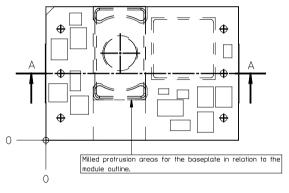
View to the left shows module from top through the coldwall showing the two areas that needs to be milled to meet the FETs for optimal heat evacuation.
