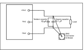
Output ripple and noise test setup
