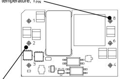
Pin 2 for measurement of maximum product temperature, T<sub>PRODUCT</sub>
