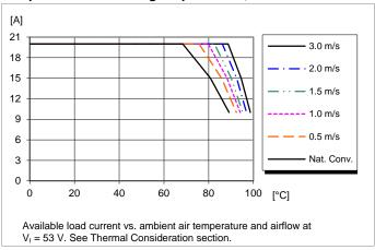
**PKU 4600E series** DC/DC Converters Input 36 - 75 V, Output up to 20 A / 66 W
