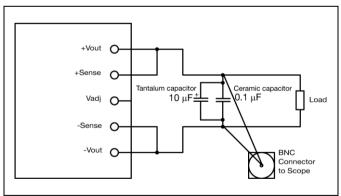
Output ripple and noise test setup
