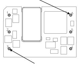
Pin 3 for measurement of minimum pin (solder joint) temperature,  $T_{\text{PIN}}$
