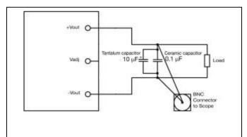
Output ripple and noise test setup
