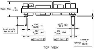
Pin positions according to recommended footprint
