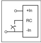
The products are fitted with a remote control function referenced to the primary negative input connection (-In), with negative and positive logic options available. The RC function allows the product to be turned on/off by an external device like a semiconductor or mechanical switch. The RC pin has an internal pull up resistor.
