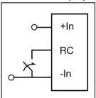
The products are fitted with a remote control function referenced to the primary negative input connection (-In), with negative and positive logic options available. The RC function allows the product to be turned on/off by an external device like a semiconductor or mechanical switch. The RC pin has an internal pull up resistor to +In.
