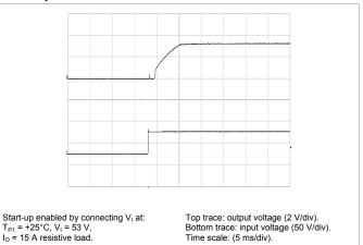
Bottom trace: input voltage (50 V/div). Time scale: (5 ms/div).
