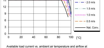
Output Current Derating, Vin=27V, test board 2
