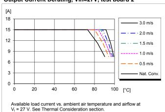
$V_1$  = 27 V. See Thermal Consideration section. Test board 1: 254 x 254 mm, 35  $\mu$ m (1 oz),8-layer test board Test board 2: 254 x 254 mm, 35  $\mu$ m (1 oz),16-layer test board
