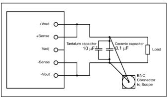
Output ripple and noise test setup
