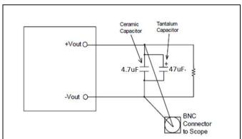
Output ripple and noise test setup
