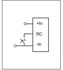
The products are fitted with a remote control function referenced to the primary negative input connection (-In), with negative and positive logic options available.The RC function allows the product to be turned on/off by an external device like a semiconductor or mechanical switch. The RC pin has an internal pull up resistor to +5 V.
