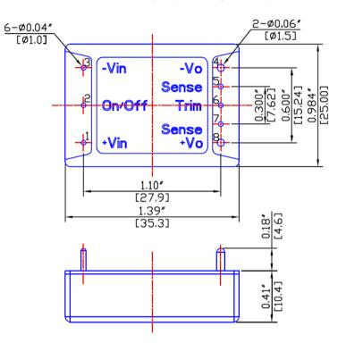
Weight : Typical 28 g. All dimensions in inches (mm). Note 1: Pin 1,2,3,5,6,7 size is 0.04±0.005 inches (1.0 mm) dia. Pin 4,8 size is 0.06±0.005 inches (1.5 mm) dia. Note 2: Tolerance .xx=±0.02" .xxx=±0.020"
