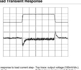
Output voltage response to load current step- Top trace: output voltage (100mV/div.). Bottom trace: load current (5 A/div.).  $T_{ref} = +25^{\circ}C, \ V_{l} = 3.3 \ V.$  Time scale: 0.1 ms/div..
