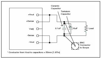
Output ripple and noise test setup
