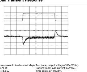
Output voltage response to load current step- Top trace: output voltage (100mV/div.). Bottom trace: load current (5 A/div.).  $T_{rel} = +25^{\circ}C, \ V_{l} = 3.3 \ V.$  Time scale: 0.1 ms/div..
