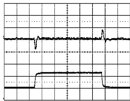
Output voltage response to load current step-
