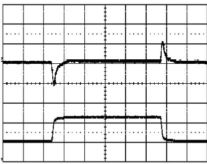
Output voltage response to load current step-
