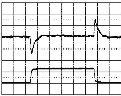
Output voltage response to load current step-
