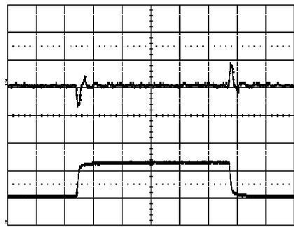
Output voltage response to load current step-change (25-50-25 A) at:
