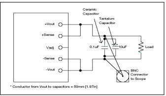
Output ripple and noise test setup
