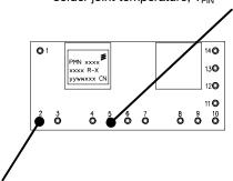
Pin 2 for measurement of maximum peak product reflow temperature, T<sub>P</sub>
