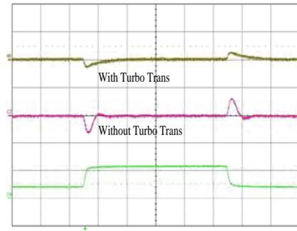
Output voltage response to load current step-change (4-12-4 A) at:  $T_{ref} = +25^\circ\text{C}$ ,  $V_I = 5\text{ V}$ .
