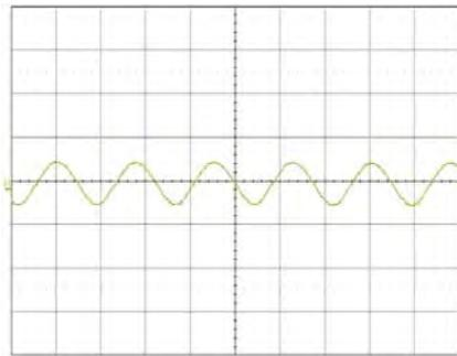
Output voltage ripple at:  $T_{ref} = +25^\circ C, V_I = 5 V,$
