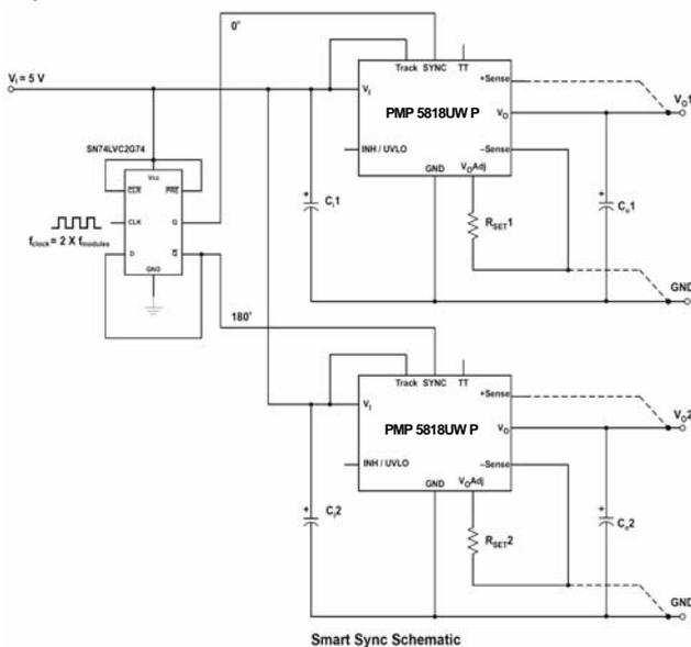
The maximum input voltage allowed for proper synchronization is duty cycle limited. When using Smart Sync, the maximum allowable input voltage varies as a function of
