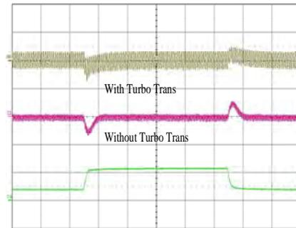
Output voltage response to load current step-change (4-12-4 A) at:  $T_{ref} = +25^\circ\text{C}$ ,  $V_I = 12\text{ V}$ .
