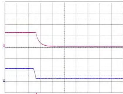
Shut-down enabled by disconnecting  $V_I$  at:  $T_{ref} = +25^\circ\text{C}$ ,  $V_I = 12\text{ V}$ ,
