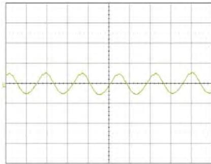
Output voltage ripple at:  $T_{ref} = +25^\circ\text{C}$ ,  $V_I = 5\text{ V}$ ,
