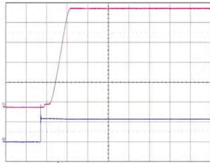
Start-up enabled by connecting  $V_I$  at:  $T_{ref} = +25^\circ\text{C}$ ,  $V_I = 12\text{ V}$ ,
