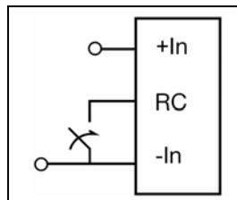
The products are fitted with a remote control function referenced to positive logic. The RC function allows the regulator to be turned on/off by an external device like a semiconductor or mechanical switch. The RC pin has an internal pull up resistor to + In.
