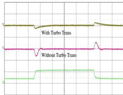
Output voltage response to load current step-change (4-12-4 A) at:  $T_{ref} = +25^\circ C, V_I = 5 V.$
