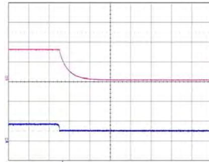
Shut-down enabled by disconnecting  $V_I$  at:  $T_{ref} = +25^\circ C, V_I = 5 V,$
