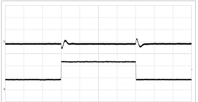
Output voltage response to load current step-change 1.5-4.5-1.5 A at: T_{P1} = +25^{\circ}\text{C} , V_I = 24\text{ V} . C_{OUT} = 2 \times 47\text{ }\mu\text{F Ceramic} + 330\text{ }\mu\text{F Polymer} Top trace: output voltage 100 mV/div. Bottom trace: load current 2 A/div. Time scale: 100 \mu\text{s} /div. Slew rate: 1A/ \mu\text{s} . 20 MHz bandwidth.
