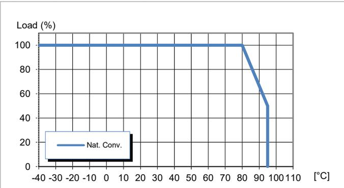
Available load vs. ambient air temperature.
