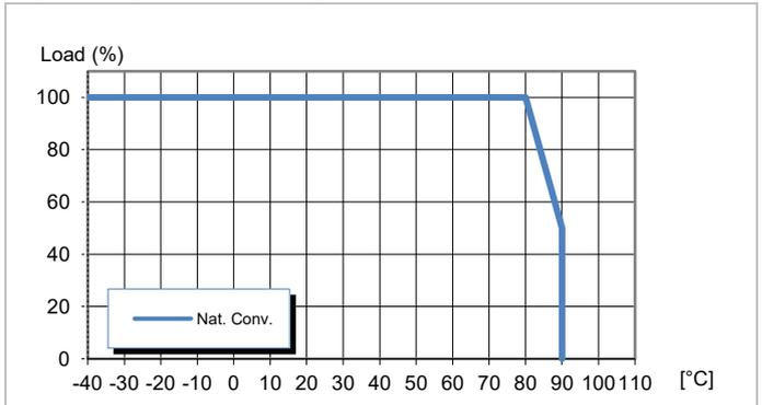
Available load vs. ambient air temperature.
