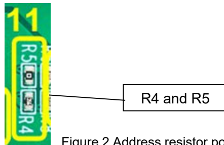
Figure 2 Address resistor position, R4 and R5, is shown in the picture.
