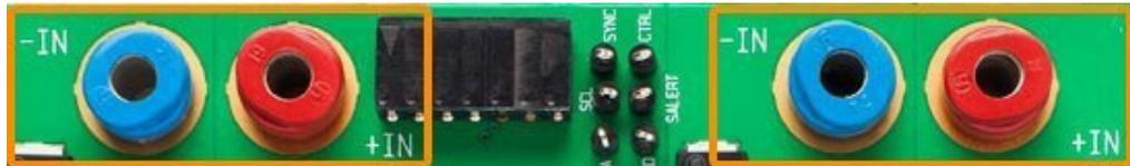
Figure 3.1a: Connect 48V between the “-IN” and “+IN” DC power connectors located on the same side of the board (see orange rectangles)
