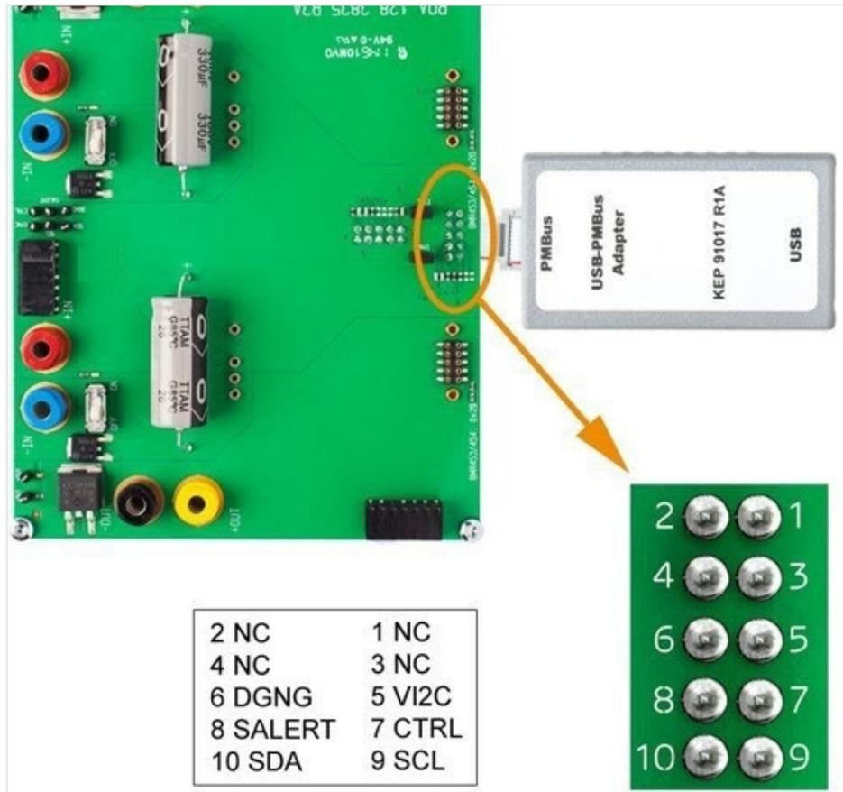
Figure 3.3a: Connection of the Flex Power Modules KE91017 PMBus-to-USB adapter (connector is found on the back side of the ROA 1283835 board)
