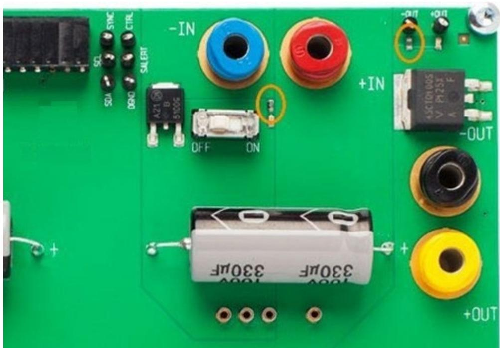
Figure 5.3: Resistors R7 and R8
