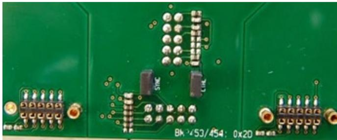
Figure 4.1: Factory default jumper settings of ROA 128 3835
