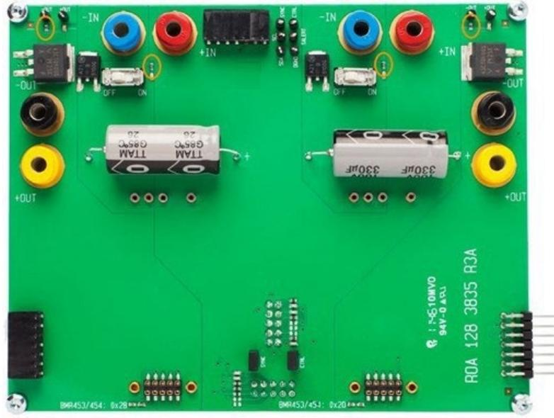
Figure 5.1: Series resistors for the LEDs
