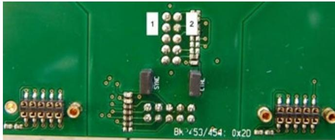
Figure 4.2: Position number of the jumpers in ROA 1283835
