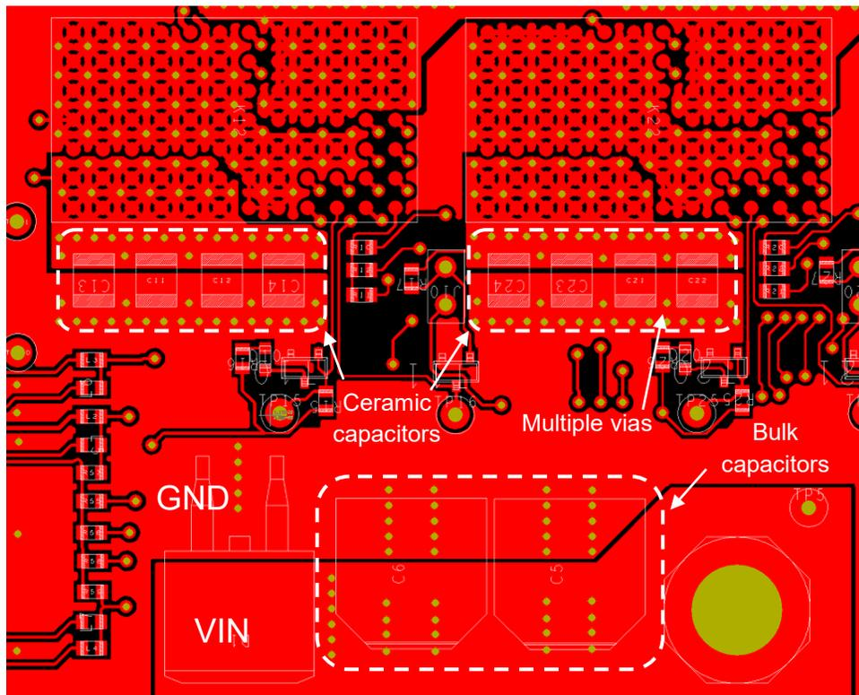
Fig 9.2 Top layer. Input capacitance in dashed areas.
