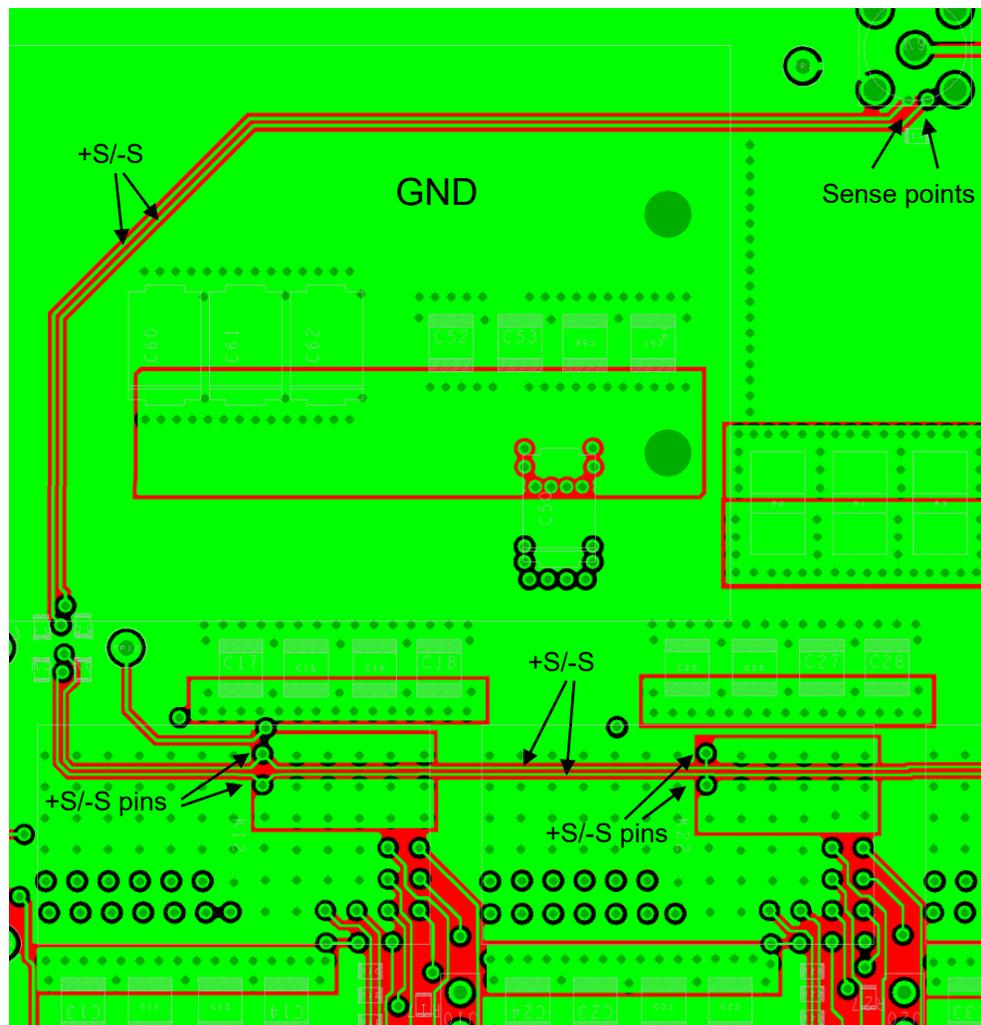
Fig 9.5 Bottom layer. Wiring of sense signals.
