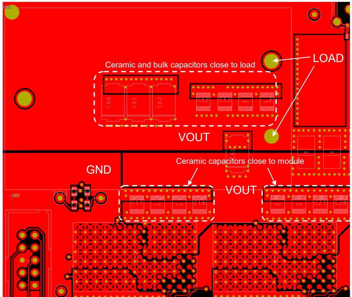
Fig 9.4 Top layer. Output capacitance in dashed areas.
